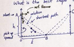
C Wart: Minimum time from A to B, powered only by gravity. Let the path between A&B be (x, y(x)). Let I[y] = total time.
